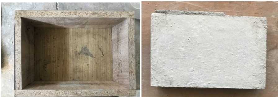
Figure III.13 : moule (3) 27.5cm × 18cm × 4cm
