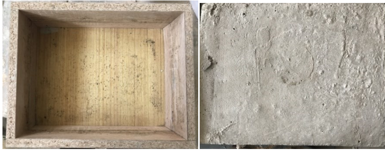
Figure III.12 : moule (2) 36cm × 27.5cm × 4cm.
