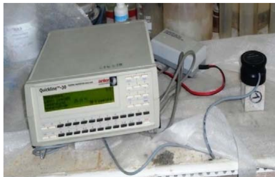
Figure IV.7 : Appareil ISOMET Quickline 30 [46]
