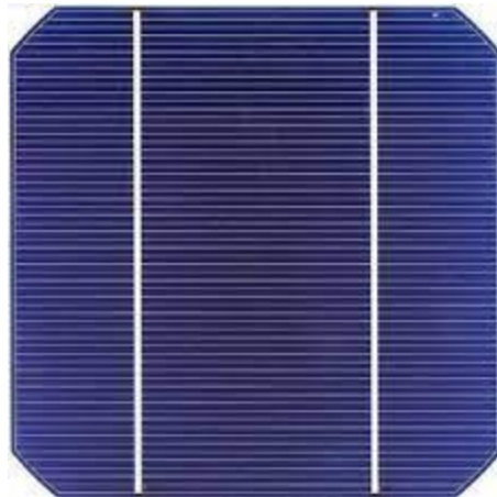
Figure I 7: cellule photovoltaïque au silicium monocristalline [8]
