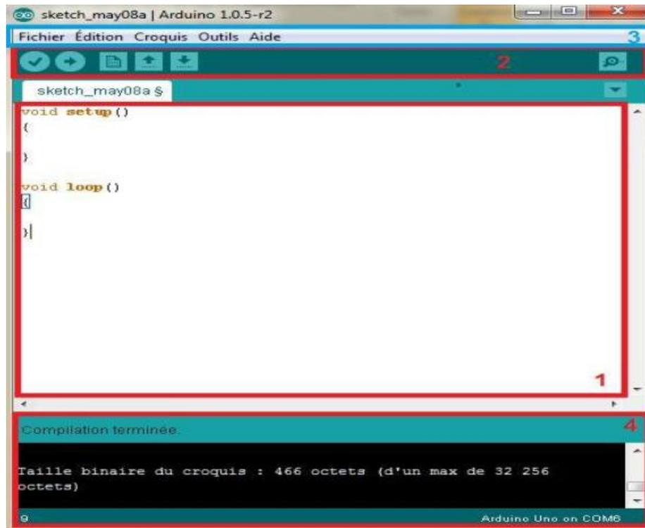
Figure 13. IDE Arduino [3]
