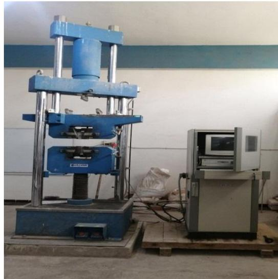
Figure III.10 : Machine traction 600 KN
