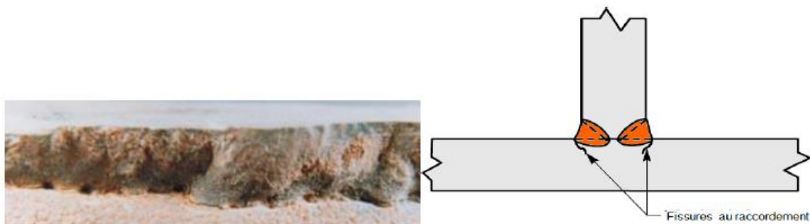
Figure II.5: fissures au raccordement.
