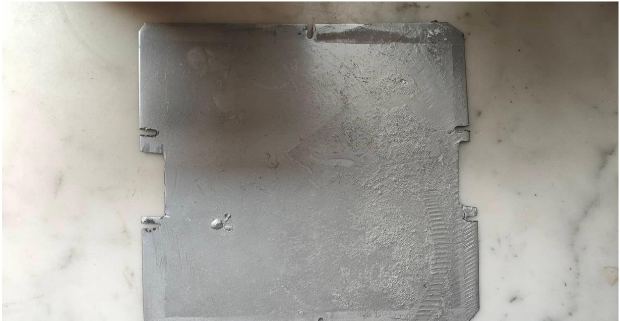
Figure 32 : Absorbeur2 plaque mince plane grise
