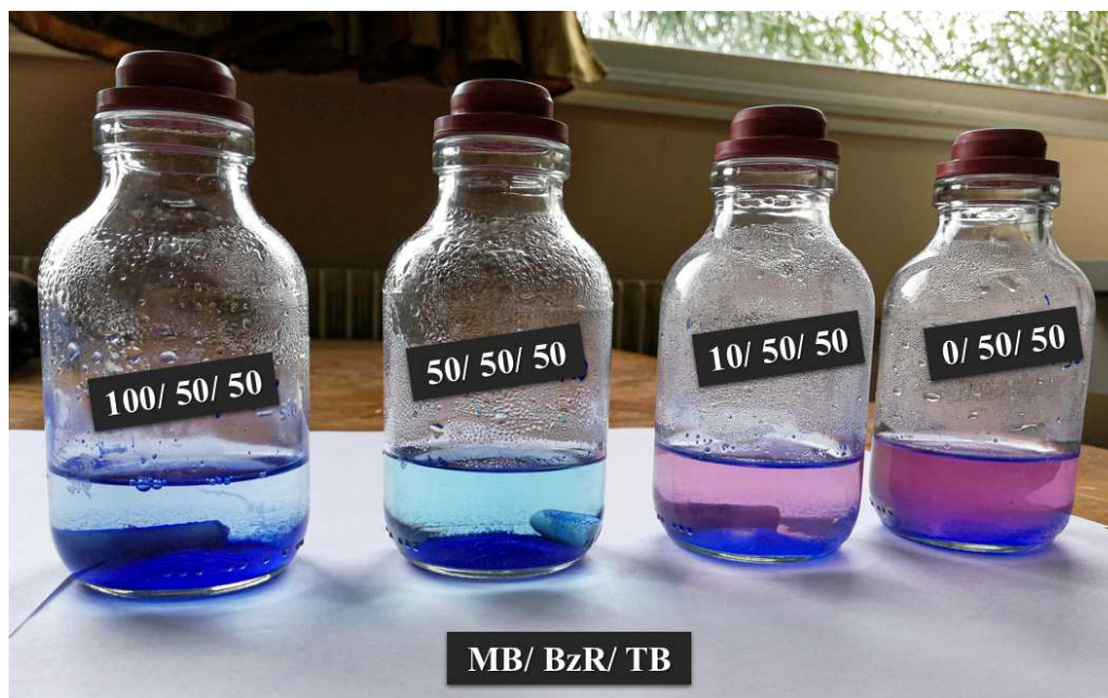
Figure 7. The solutions obtained after adsorption at different concentrations of Methylene Blue.
