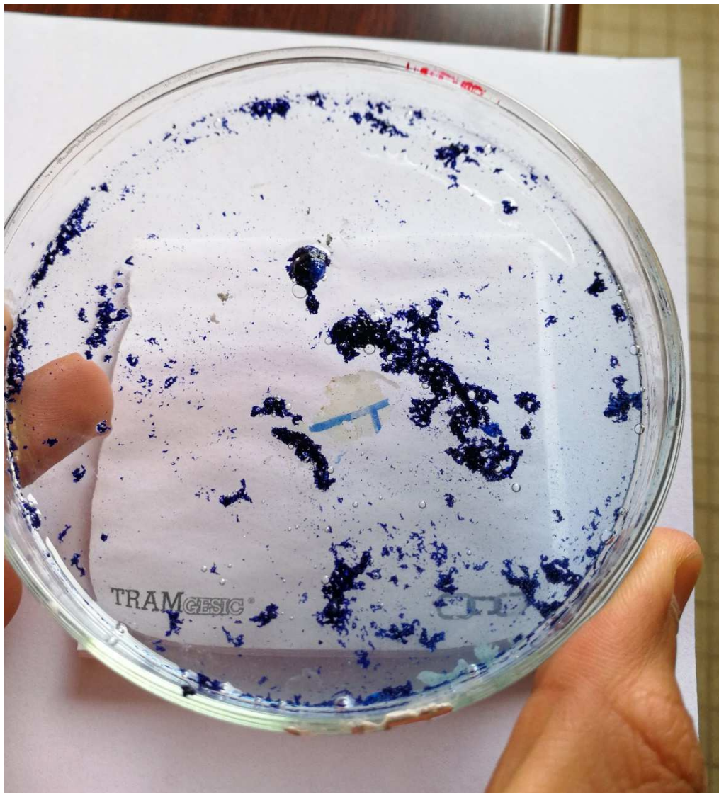
Figure. 18. The physical state of the macro-flocs formed at the end of adsorption.
