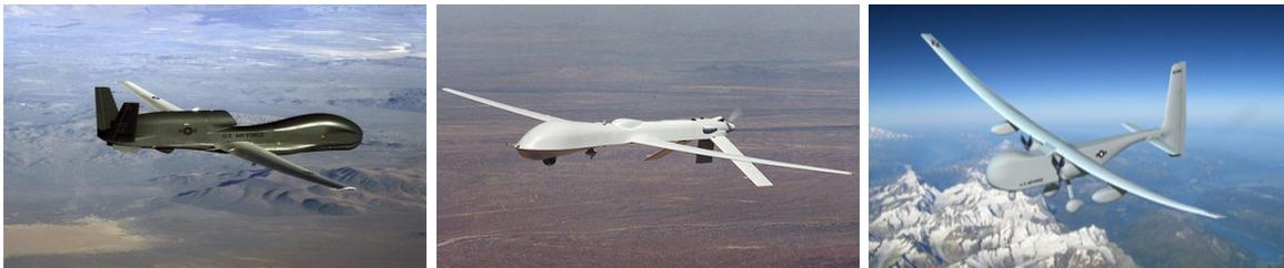
FIGURE 1.2 – HALE et MALE : (a) RQ-4 Global Hawk - (b) MQ-1 Predator - (c) Orion.
