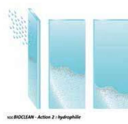
Figure 108 BIOCLEAN action 2 hydrophilie
