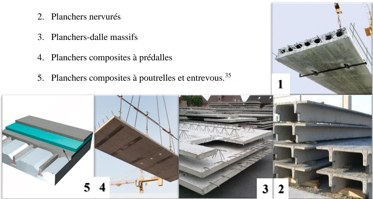
Figure 38. Exemples des planchers.
