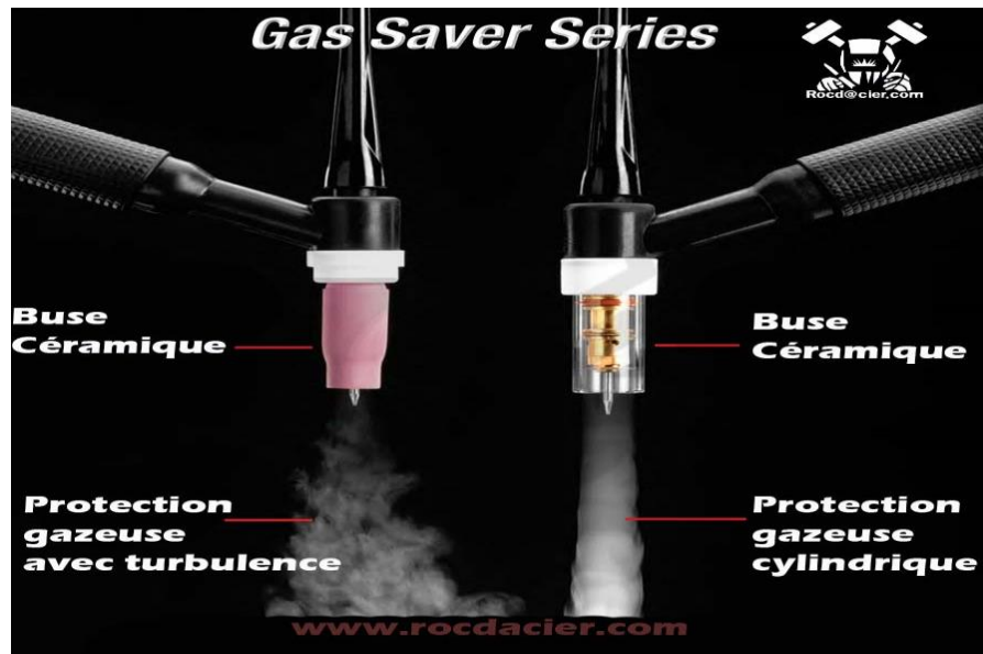
Figure II. 2 Avantages buses pyrex TIG [25]
