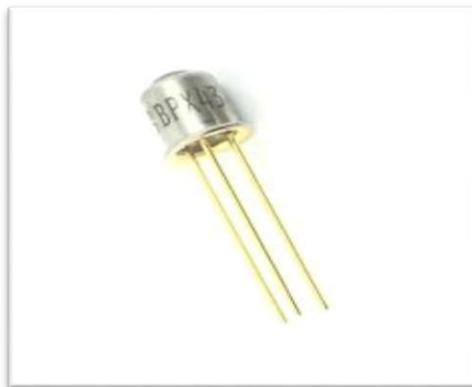
Figure 2.3. Le phototransistor bpx43.
