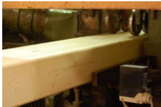
Figure 29: Rabotage des quatre faces.
