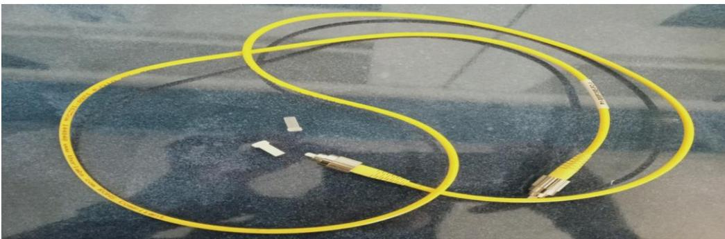
**Figure III.1:** Fibre optique monomode P1-SMF-28-FC-1(thorlabs)
