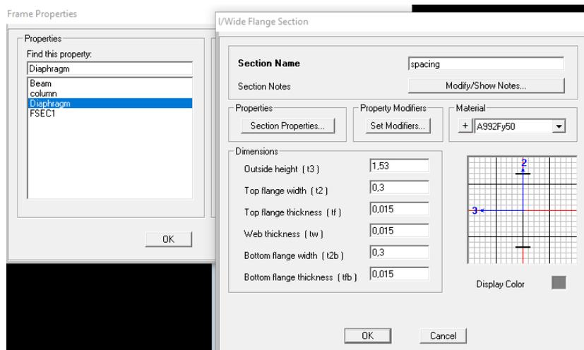
figure 4. 9: definition of dimensions of the steel beam spacing
