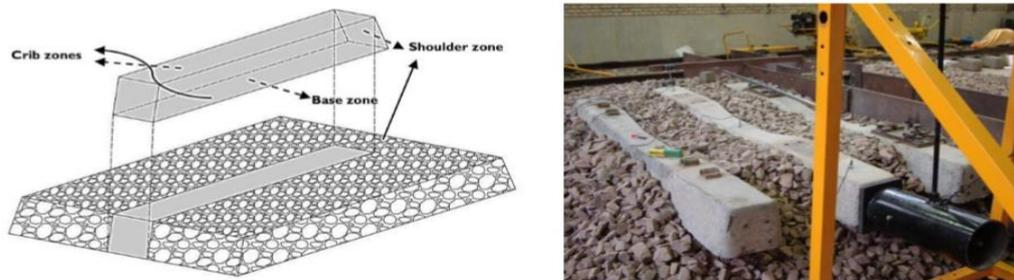
figure 2. 33: Base, crib and shoulder zones and Test setup apparatus (Morteza E. and Ahmad H., 2019)
