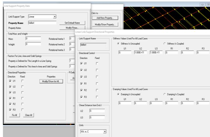
figure 4. 13: definition of ballast stiffness
