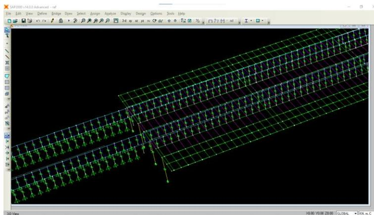
figure 4. 28: creation of the sleepers, rails, and ballast
