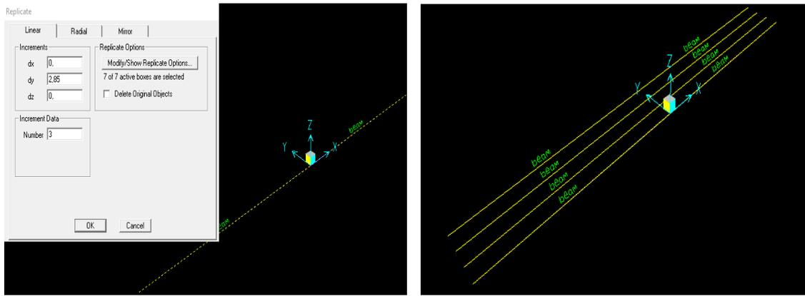
figure 4. 17: replication of the beams
