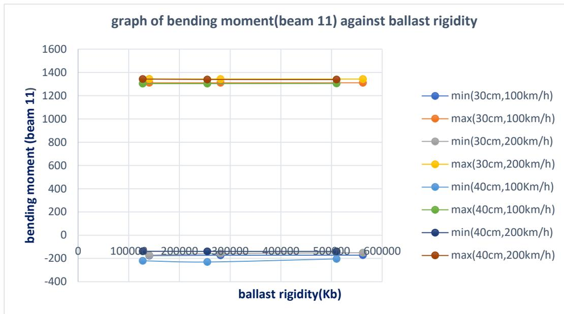
figure 5. 10: Variation of bending moment of mid-span steel beam and ballast rigidity
