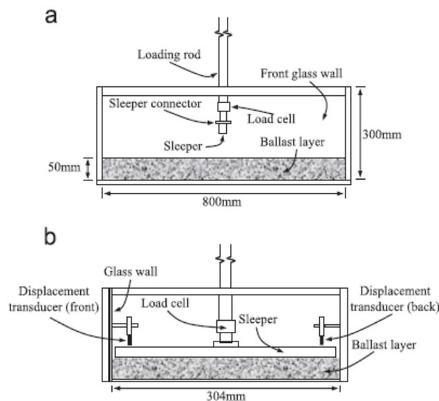
figure 2. 26: Sandbox experiment (*Soils and Foundations 2016;56(4):652–663*)
