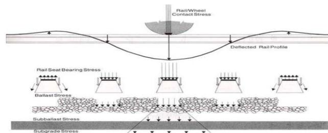
**figure 2. 32: Typical wheel load distribution in track (Selig and Waters, 1994)**
