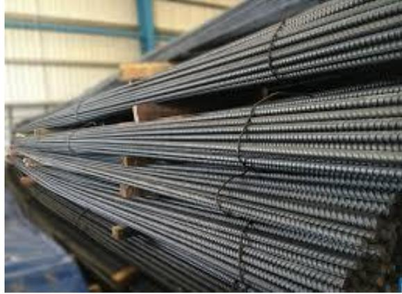
figure 3. 6: Steel re-bars (The constructor, 2009)
