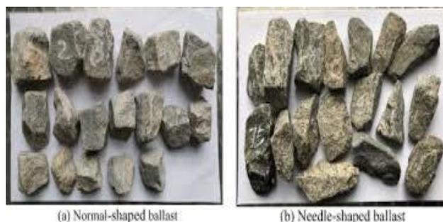
**figure 2. 20: Ballast of different angularity and shape**
