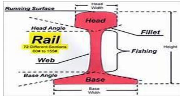
figure 2. 5: Different parts of a rail (Slide share, 2015)
