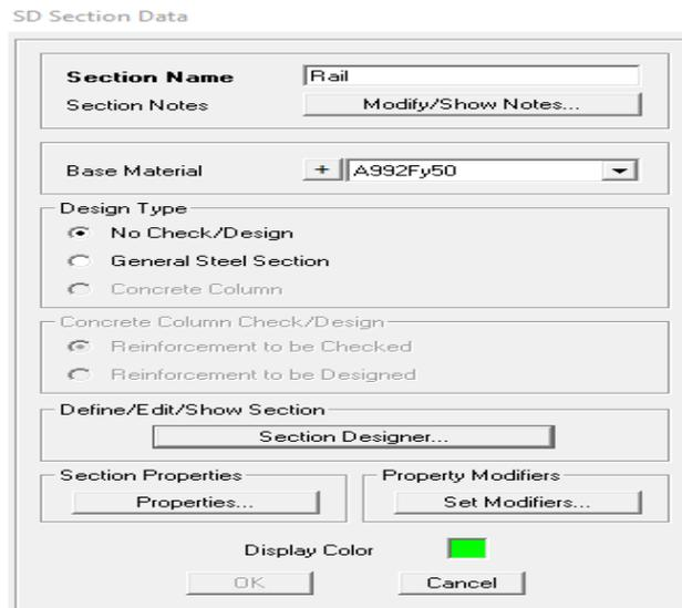
figure 4. 15: Defining of the section rail and selecting the section property
