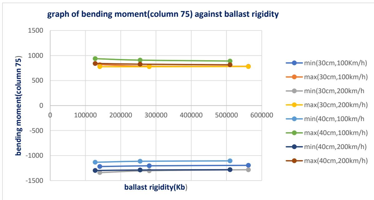
figure 5. 9: Variation of the bending moment of column 75 and ballast rigidity (Kb)
