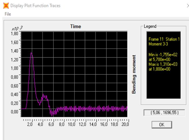
figure 5. 5: graph of central beam bending moment against time
