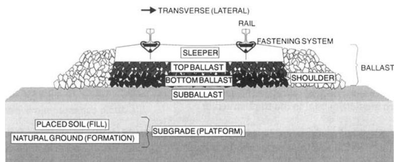
figure 2. 16: *Cross section view of the ballast track. (Selig & Waters, 1994). (Lim, Wee Loon (2004) Mechanics of railway ballast behaviour. PhD thesis, University of Nottingham.)*
