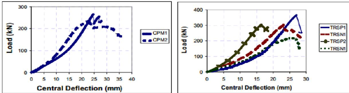
figure 2. 10: Load-deflection of CPM, TRSP and TRSN test,( Siti, 2008)
