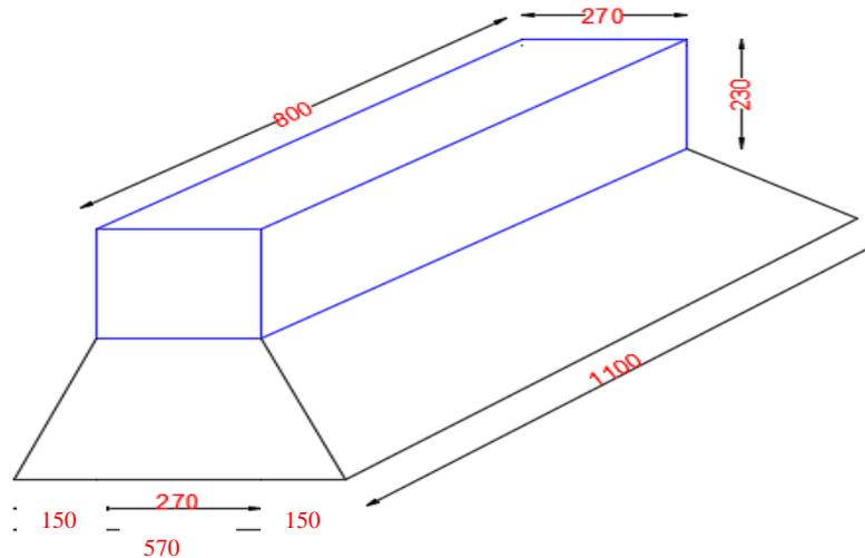
figure 4. 12: dimensions of the sleeper and that of ballast
