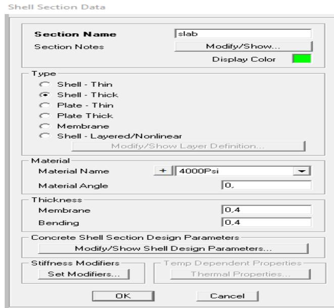
figure 4. 10: definition of the slab dimensions
