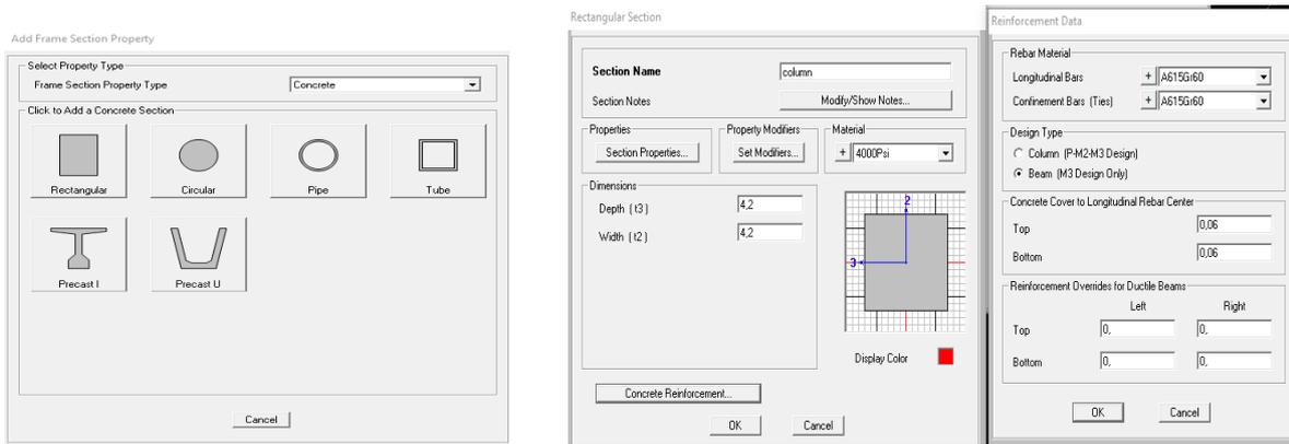
figure 4. 7: windows from which the column material property(left) and section(right) is defined
