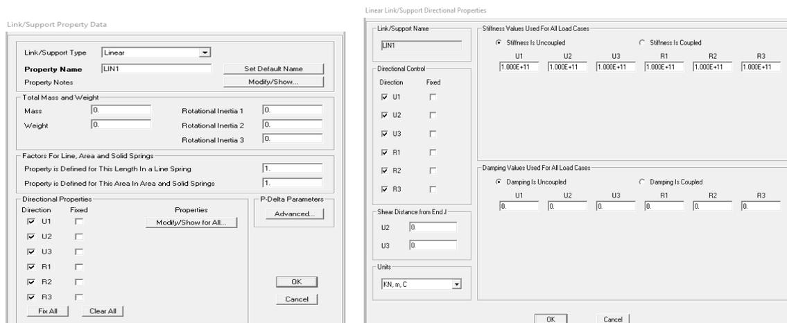
figure 4. 22: Defining the stiffness of the link supports
