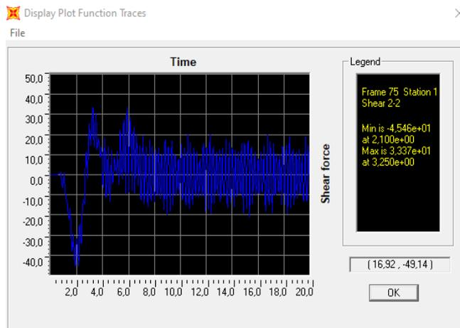
figure 5. 3: graph of shear force against time
