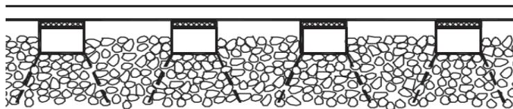
**figure 2. 31: Load distribution region in continuous granular ballast(W.M.Zhai, K.Y.Wang, J.H.Lin, 2014)**
