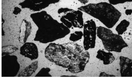
**figure 2. 19: Examples of granite/ syenite ballast of thin sections.**( Railway Geotechnics, Dingqing Li, James Hyslip, Ted Sussmann, Steven Chrismer)
