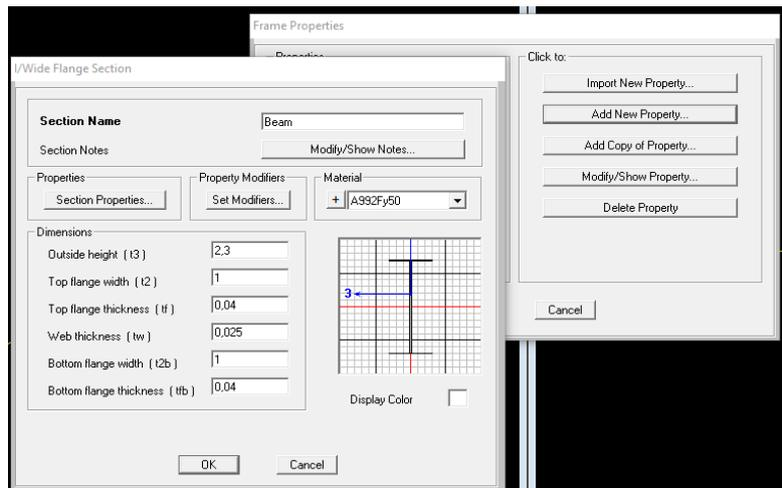
**figure 4. 6: window displaying the definition of the beam section.**
