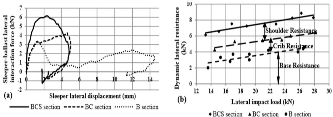
figure 2.34: Sleeper ballast lateral and Dynamic lateral ( Morteza et al., 2016)
