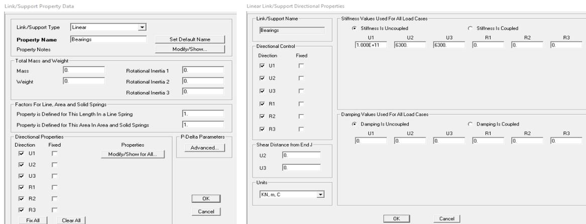
figure 4. 23: definition of bearing stiffness
