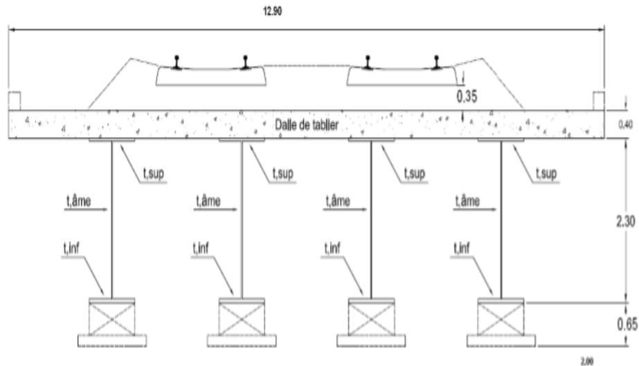
figure 3. 2: Transverse view of the deck section.
