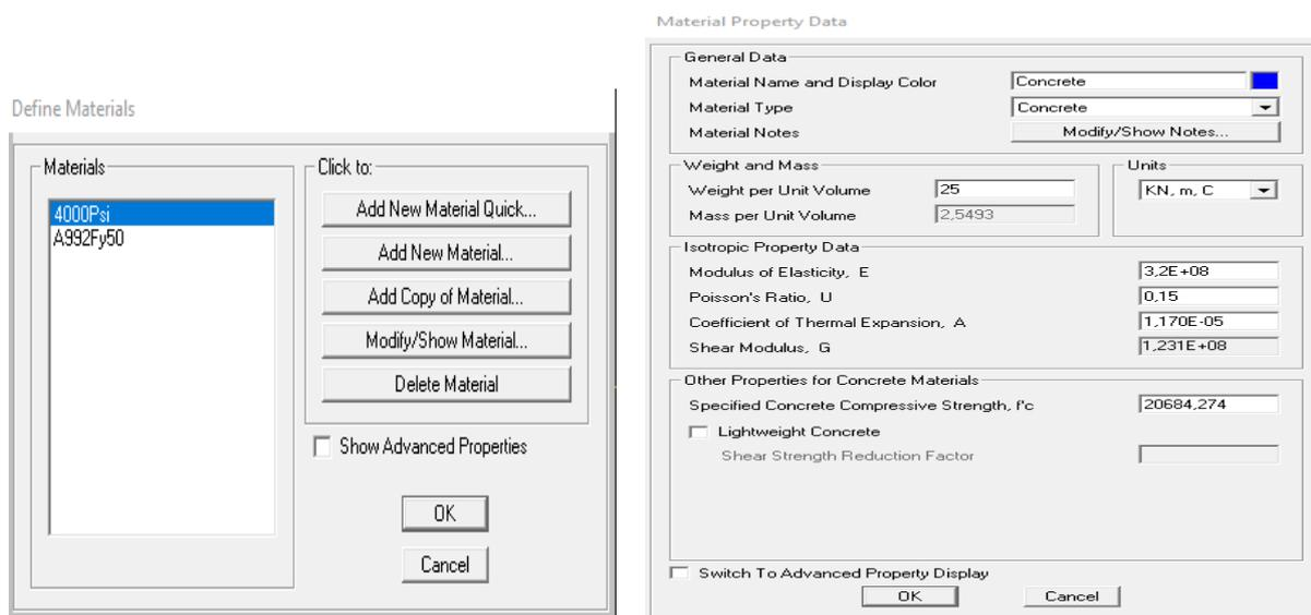
figure 4. 3: windows displaying concrete property definition
