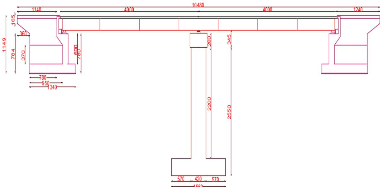
figure 3. 1: longitudinal view of the railway bridge
