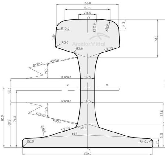
figure 3. 7: section steel track rail (ArcelorMittal,2012)
