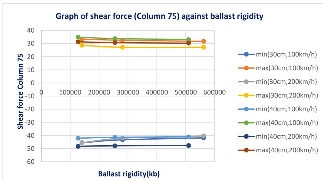
figure 5. 8: Variation of the shear force and the ballast rigidity
