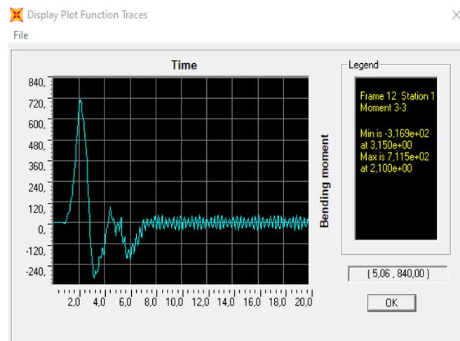
figure 5. 6: graph of joint beam bending moment against time
