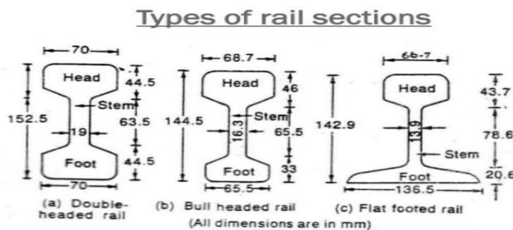
figure 2. 6: Types of rail sections ( Slideshare, 2014)
