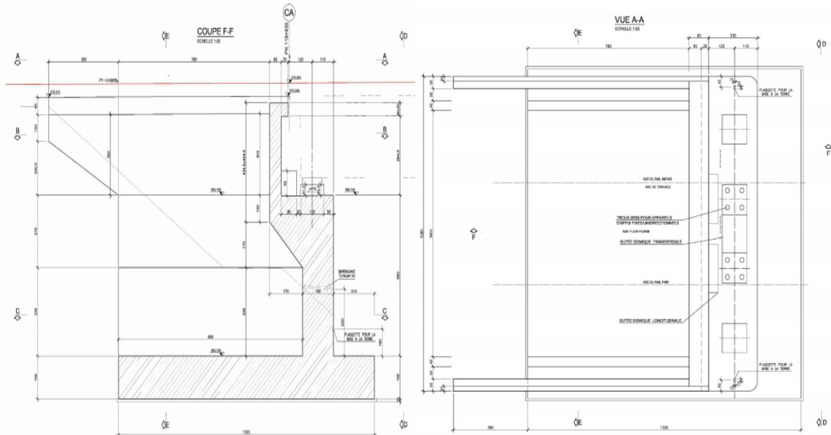
figure 3. 12: Abutment sections
