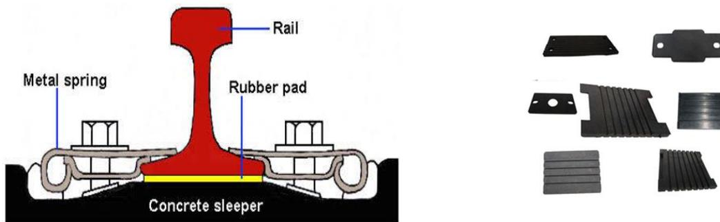
**figure 2.7 : Rail fastening and different kinds of rail pads (Malysian Rubber Board, 2002)**
