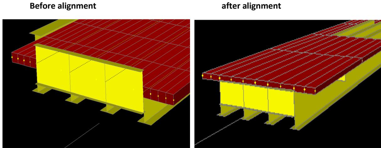
figure 4. 21: alignment of the steel beams and steel beam spacing with the slab section
