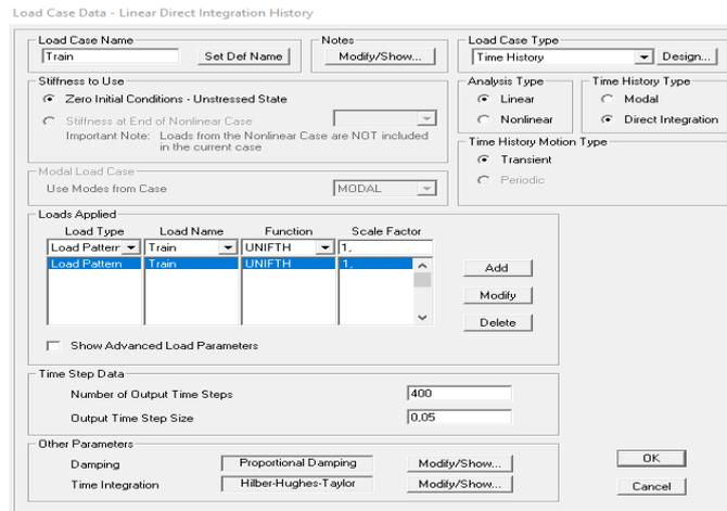
figure 4. 34: definition of the train load case
