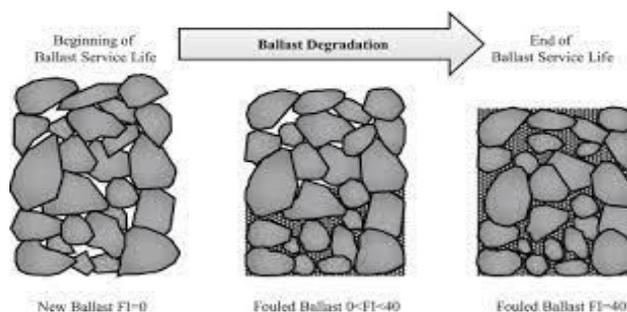
figure 2. 23: Cycle of ballast degradation(Raymond and Diyaljee, 1979, Railroad ballast load ranking classification)
