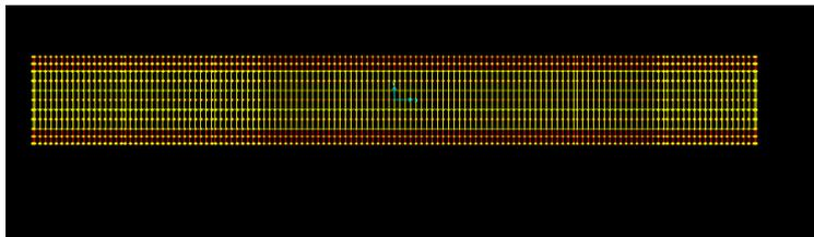
figure 4. 27: creation of nodes of 60cm apart from each other on the area section
