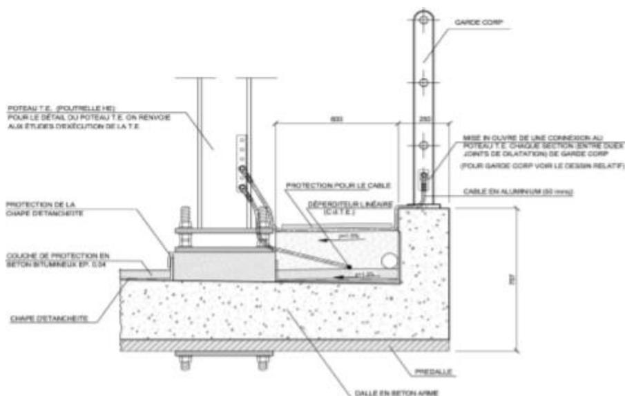
figure 3. 14: construction *detail of the anchoring system.*
