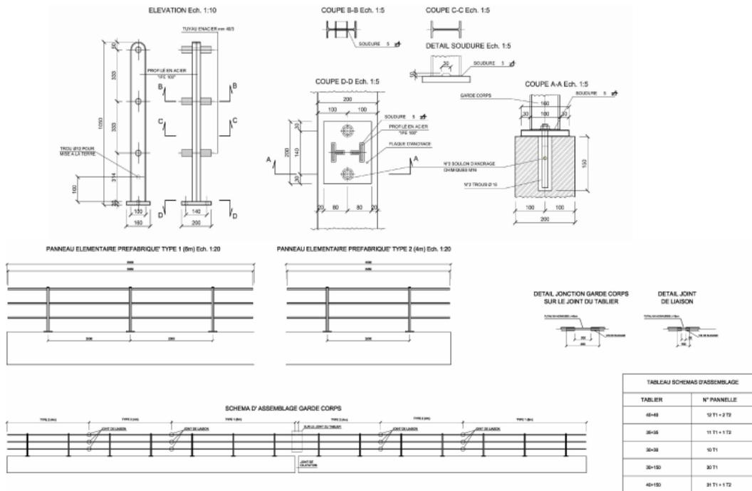
figure 3. 13: plan of the security *barriers*
