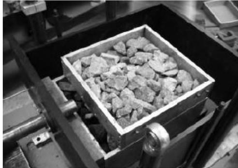
**figure 2. 21: Direct shear test experiment.**( Railway Geotechnics, Dingqing Li, James Hyslip, Ted Sussmann, Steven Chrismer)
