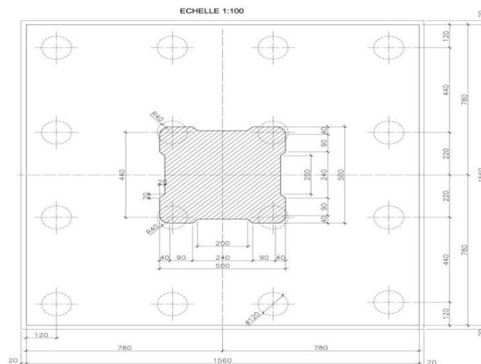
figure 3. 11: Foundation of the column(P01)
