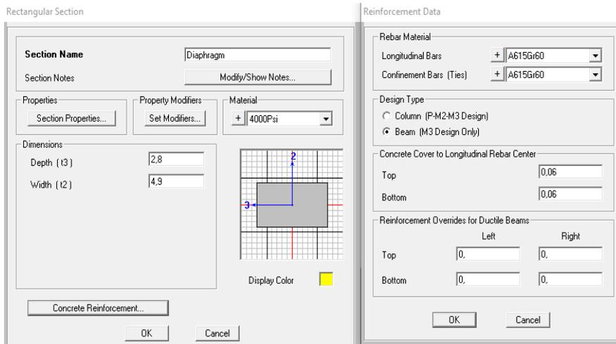
figure 4. 8: windows displaying the definition of the diaphragm section.
