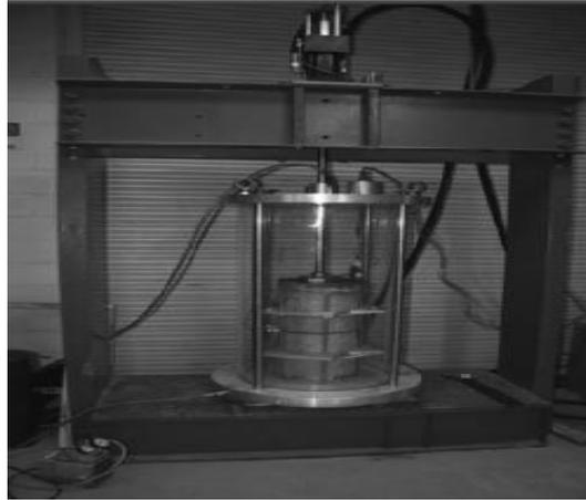
figure 2. 22: Large (0.3 m, 12 in. diameter) triaxial test apparatus. (Courtesy of University of Illinois Urbana-Champaign, Champaign, Illinois.)
