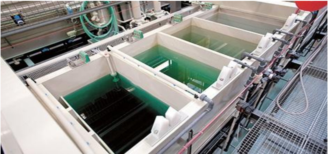
Figure 30: Bains de phosphatation. (Metrohm )
