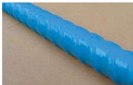
Figure 1.7: Revêtement anticorrosion [ERSIGROUP, 2017]
