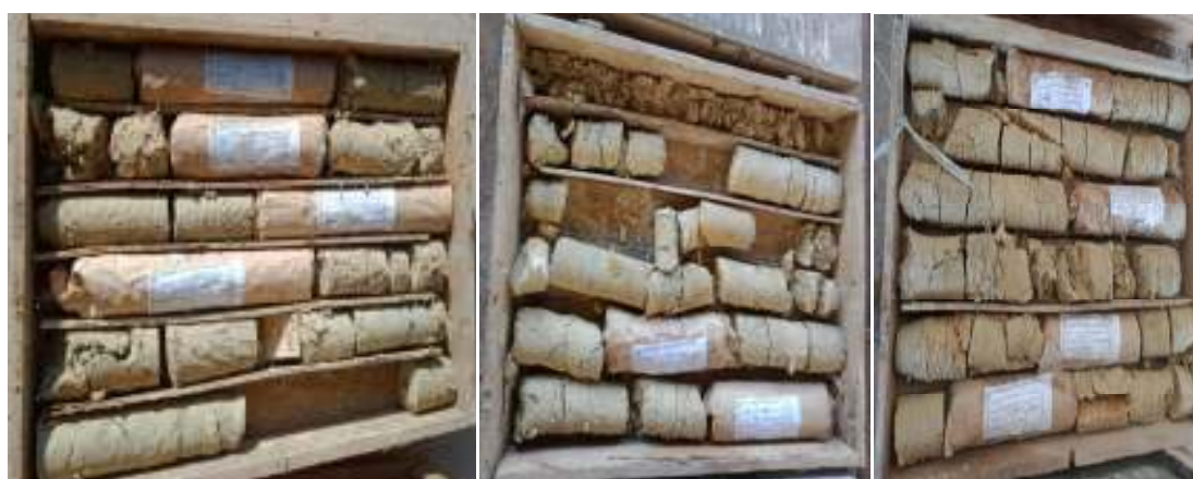
Figure (4.38): Caisses de sondage SC3
