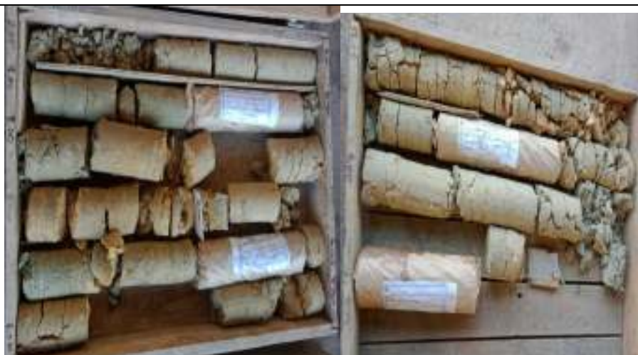
Figure (4.37):Caisses de sondage SC2
