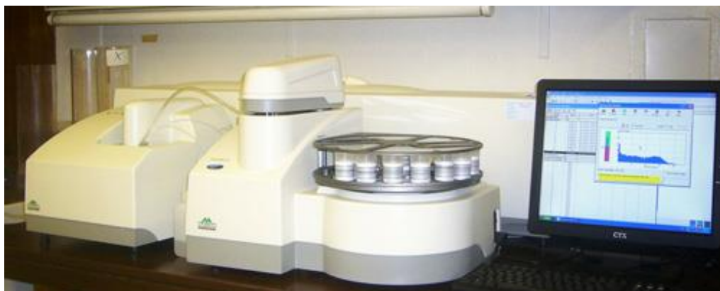
Figure 2.3 : Mastersizer 2000 (Malvern Panalytical, [7])
