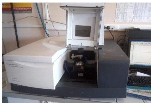
**Figure II.5.** Appareil FTIR Agilent Technologies Cary 600 series.
