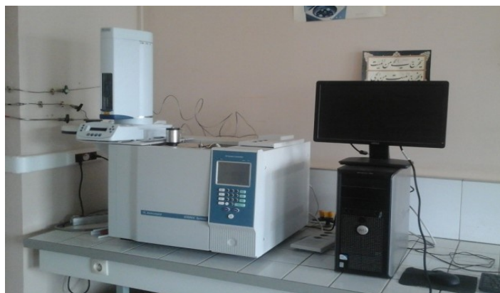
Figure II.19 : Appareil de chromatographe en phase gaz (CPG) (YOUNGLIN (YL Instrument 6500GC System)).
