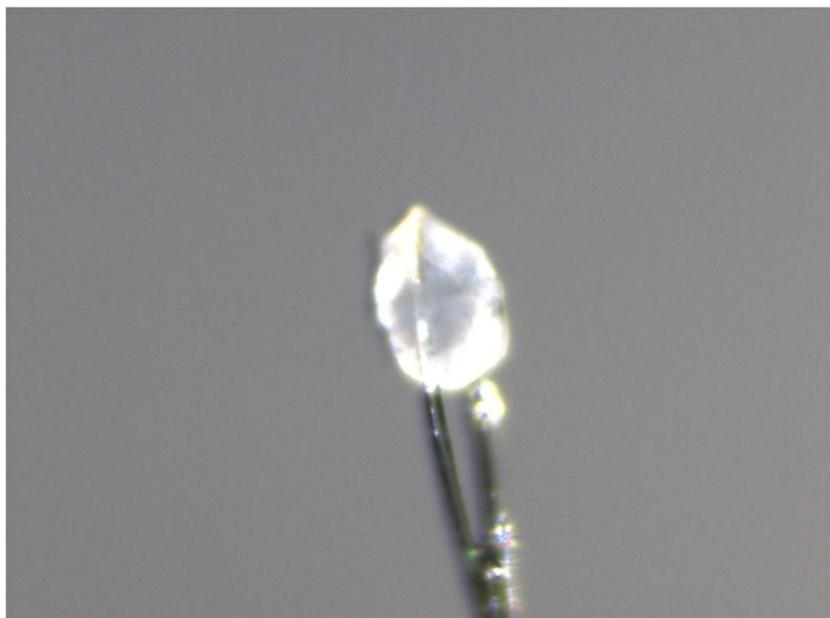
**Image 1.** Cristal de  $[[\text{Al}(\text{dpa})_2] (\text{NHEt}_3)]$
