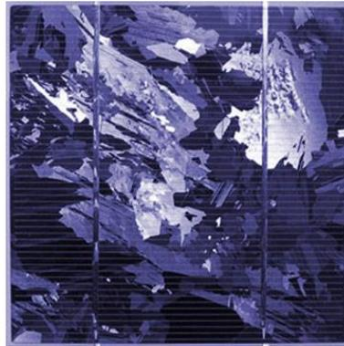
**Fig. I.19 :** Cellule photovoltaïque polycristalline [4]
