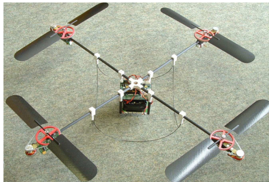
FIGURE 1.17 – Le Quadrirotor OS4
