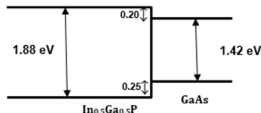
Figure 1. Block band diagram InGaP/GaAs [6]
