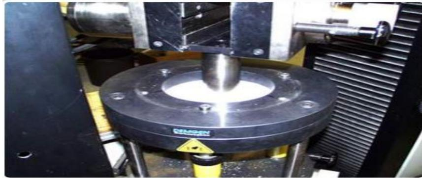
Figure 1-24 Essai de perforation statique (CBR)
