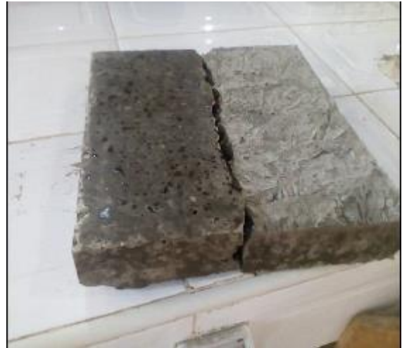
Figure IV-5: Eprouvettes (27x13x4) (Hamou, 2019)
