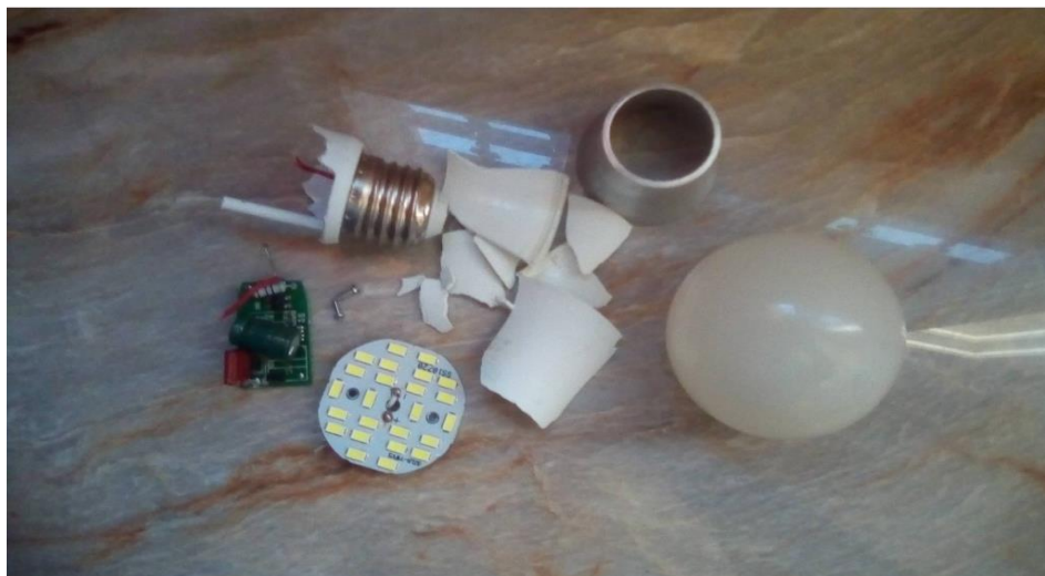
Figure 4.2. Composants de lampe LED
