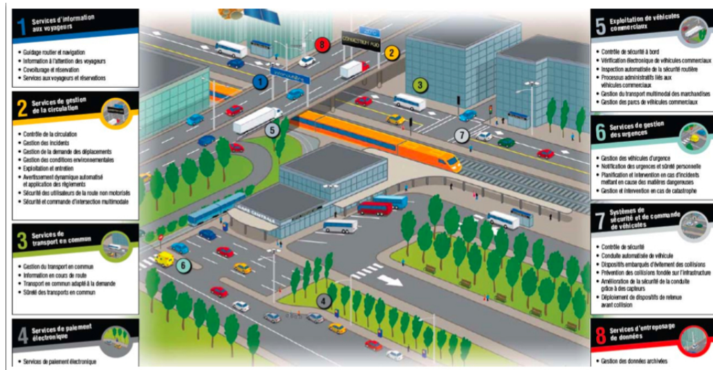
Figure 1.4: Architecture générale d'un ITS
