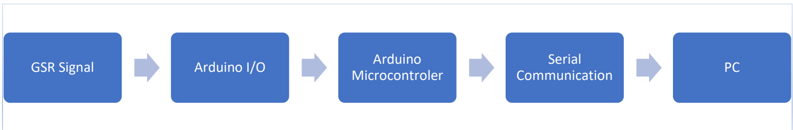
Figure III-15: Block diagram of the GSR signal acquisition.
