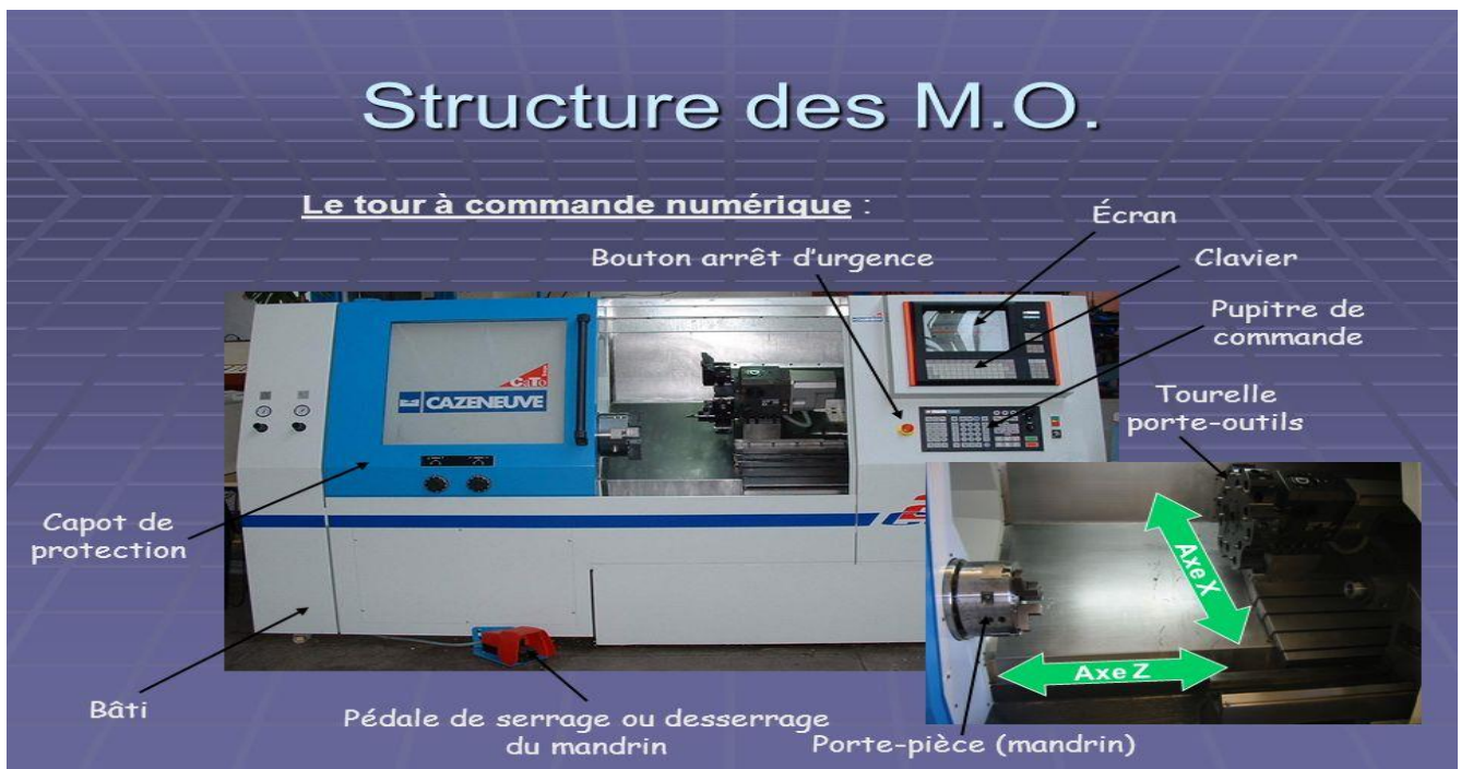
Figure II .1: Structure des MO.
