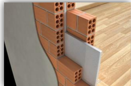
Figure 126: Mur double paroi
