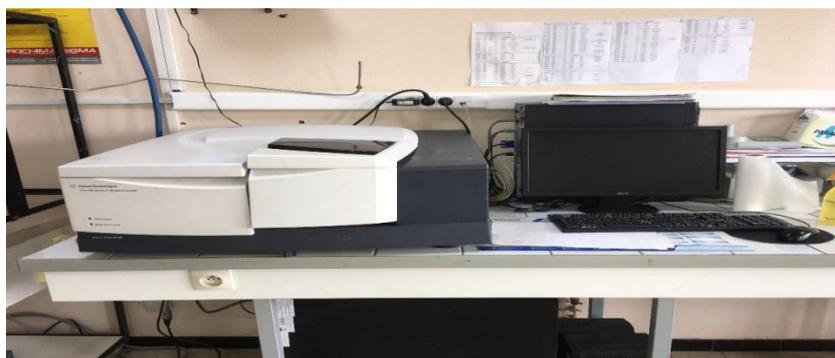
**Figure 3** : Appareil FTIR Agilent Technologies Cary 600 series
