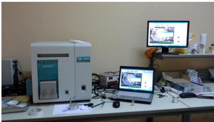
Figure 6 : HITACHI-TM-1000 Tabletop Microscope
