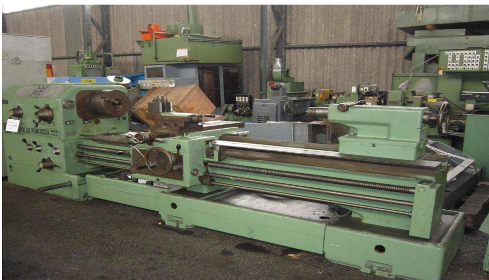
Figure II.12 Machine a outil (tour).
