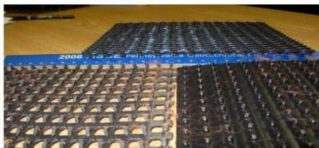
(c) Other geonets (boxshaped channels and protruding columns)
