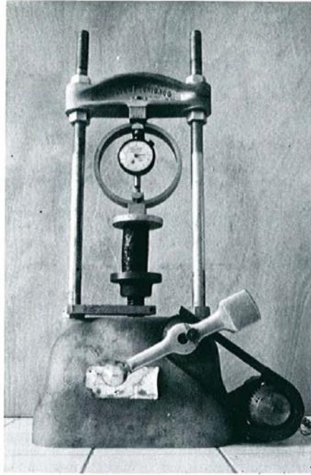
Figure 4.14 Essai de compression simple [36].
