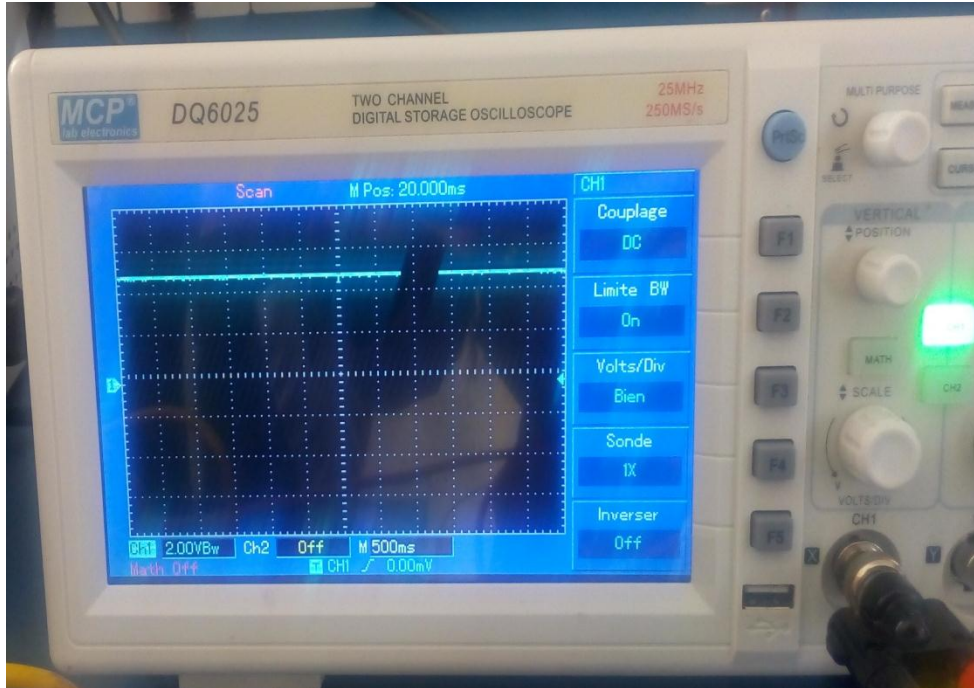
Figure III.7 : test de circuit alimentation (5V).
