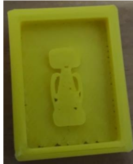
Fig30. The negative mold of ears diffuser/nozzle structure.
