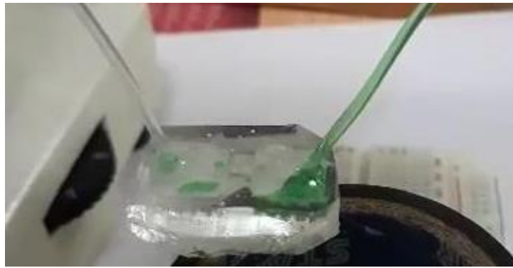
Fig 33. Testing the simple diffuser/nozzle structure.
