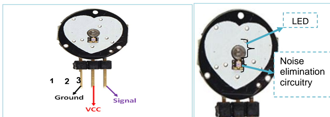
Figure (21): Heart Rate sensor Pinout
