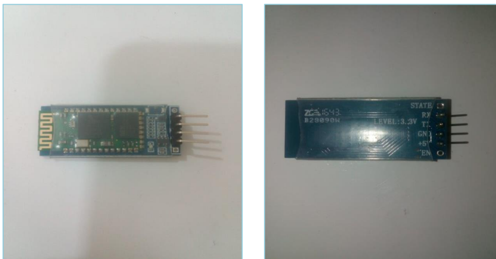
Figure (5): The HC-06 Bluetooth module
