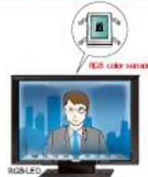
The RGB color sensor detects the white balance of LCD backlight optical waveguides and controls the light level of each RGB LED to stabilize the LCD backlight color.
