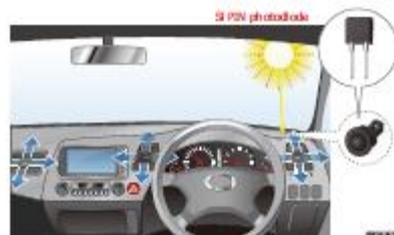
Si photodiodes are used to detect the amount of sunshine to control the volume of air flow for automotive air conditioners.
