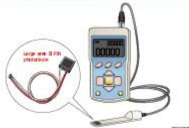
Large area type Si PIN photodiodes are used to measure the light levels of various light sources such as laser diodes and LEDs.
