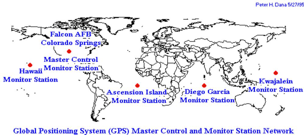
**Figure II.11:** Global Positioning System (GPS) Master control and Monitor Station Network
