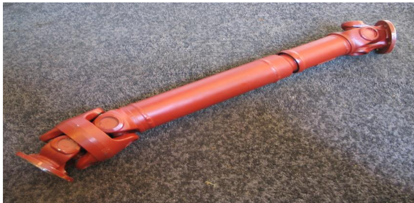
Figure I.1 :Arbre de transmission
