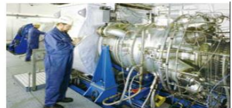
SGT-400 core engine test facility.
