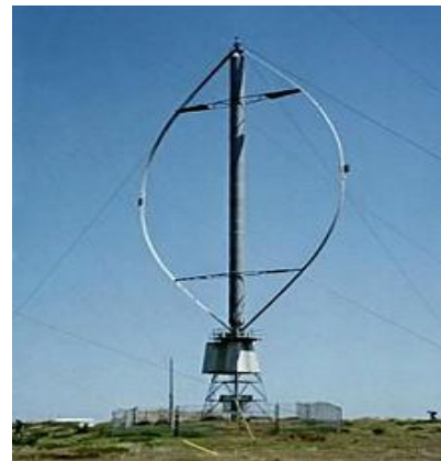
Figure. I. 3. Rotor de Darrieus [7]
