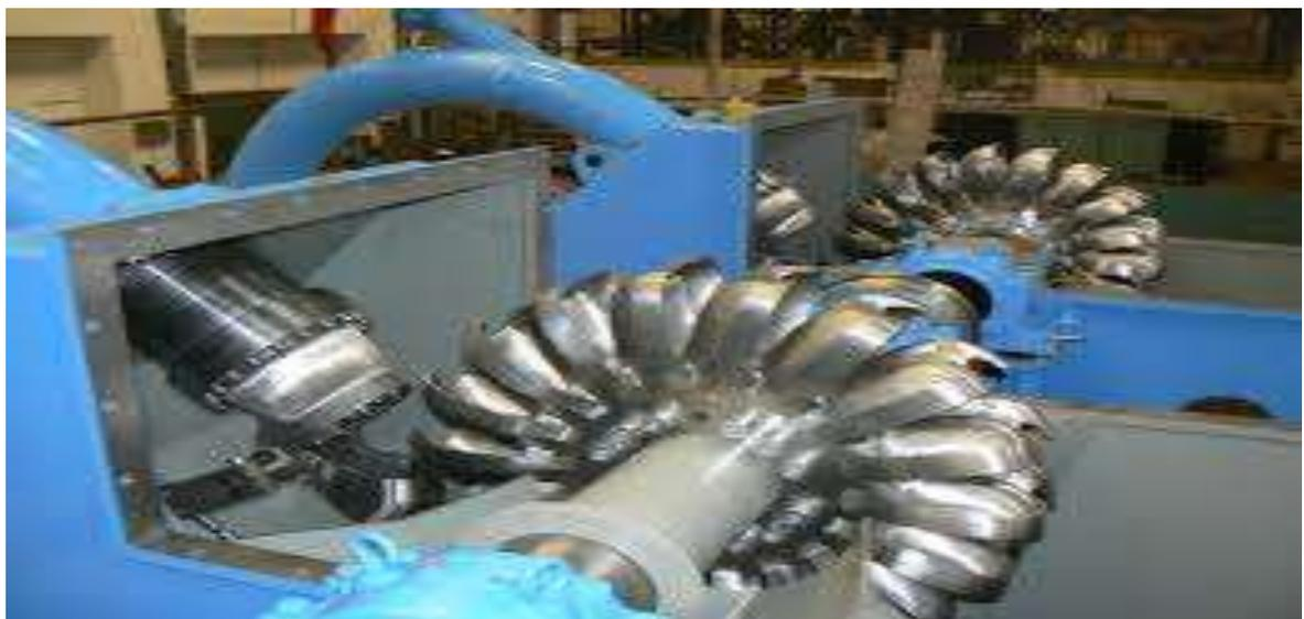
**Figure (II.2) :** Turbine Pelton
