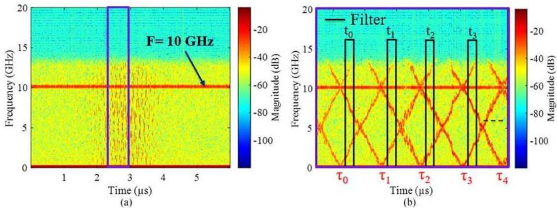
Fig. 3. (a) Spectrogram of the beat signal. (b) Zooming in. The spectrogram shows the instantaneous beat frequency. The repetition rate  $F = 10$  GHz can be deduced from (a). The beat signal will be filtered out at every time corresponding to an instantaneous frequency lower than half the repetition rate as shown in (b) (black).
