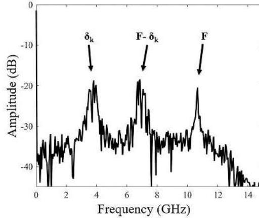
Fig. 4. RF beat spectrum of the filtered signal  $Sig_k$ .  $\delta_k$  and  $F - \delta_k$  are the beat frequencies between the swept source and the  $k$ th and  $(k + 1)$ th modes respectively.  $F$  is the repetition rate.
