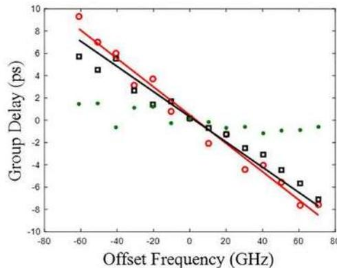
Fig. 7. Group delay measured directly at the filter output (red circles), after 100 m of SMF (black squares), linear fit (red line), predicted group delay after 100 m of SMF using 17 ps/nm.km of dispersion (black line). The standard error is less than 1.5 ps (green dots).
