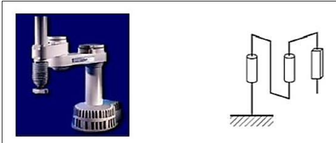
Figure II.20. Structure d'un robot SCARA
