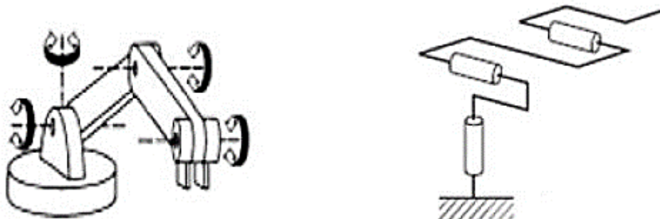
Figure II.21. Structure d'un robot 3R
