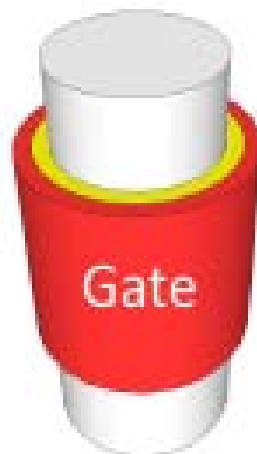
Figure 2-19 : Cylindrique GAA MOSFET.
