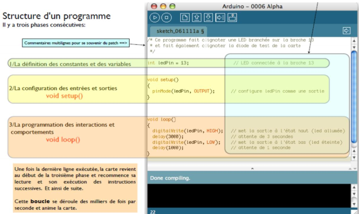
Figure II-23 Structures de programme Arduino
